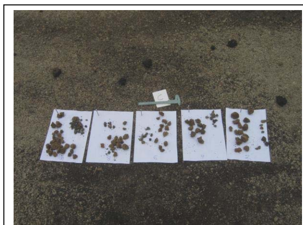
Fig. 14. Example of sampling an unspecified area of section C in different time steps: 2, 4, 8 and 15 minutes (from right to left).
